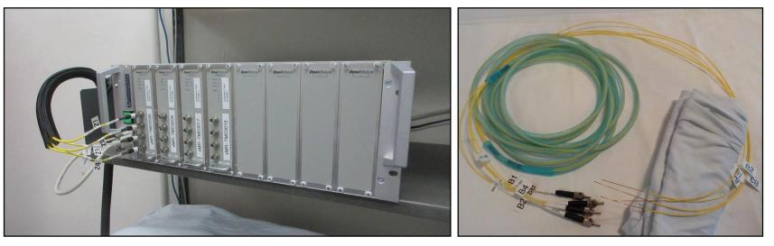
Figure 3: Omniflex temperature system (left) and T1C fiber optic temperature probes (right) [4].
